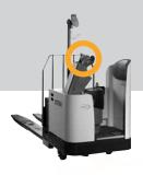
**REAR DIRECTIONAL STEERING (Sometimes called Reverse Steering.)**Shows direction truck will turn when steering handle is turned clockwise.
