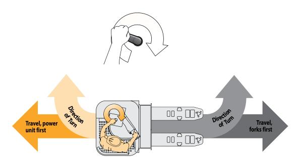
**PRONT DIRECTIONAL STEERING (Sometimes called Forward Steering.)**Shows direction truck will turn when steering handle is turned clockwise.
