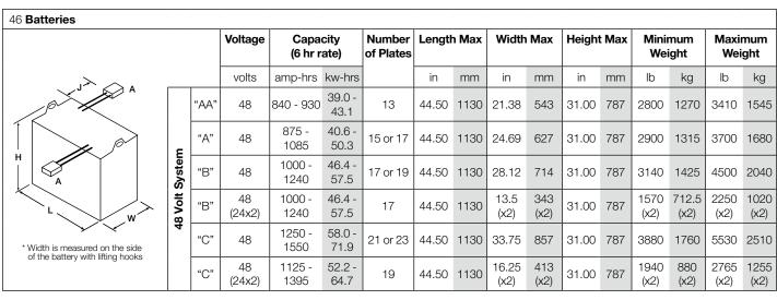
Connector Location / Length (J) is A/15" (A/381 mm). Standard Connectors: 48 Volt "AA", "A", "B", "C" = SB350 Blue; 48 (24x2) Volt "B", "C" = SB350 Red.
