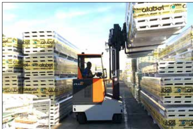
FLUXX - up to 8,800 lbs | up to 295" lift height
