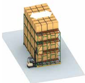
Push-Back Rack First-in, last-out Variable truck and aisle
